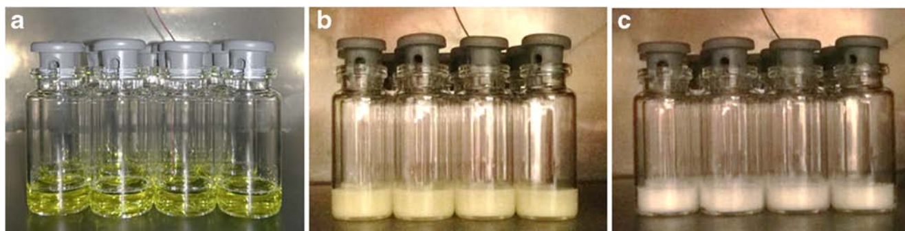
Fig. 2 Photograph of: (a) prelyo solution at RT, immediately after loading into the freeze-dryer. (b) Frozen solution - before annealing. (c) Frozen solution - after annealing.
